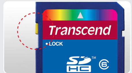
Mechanical write-protection switch
